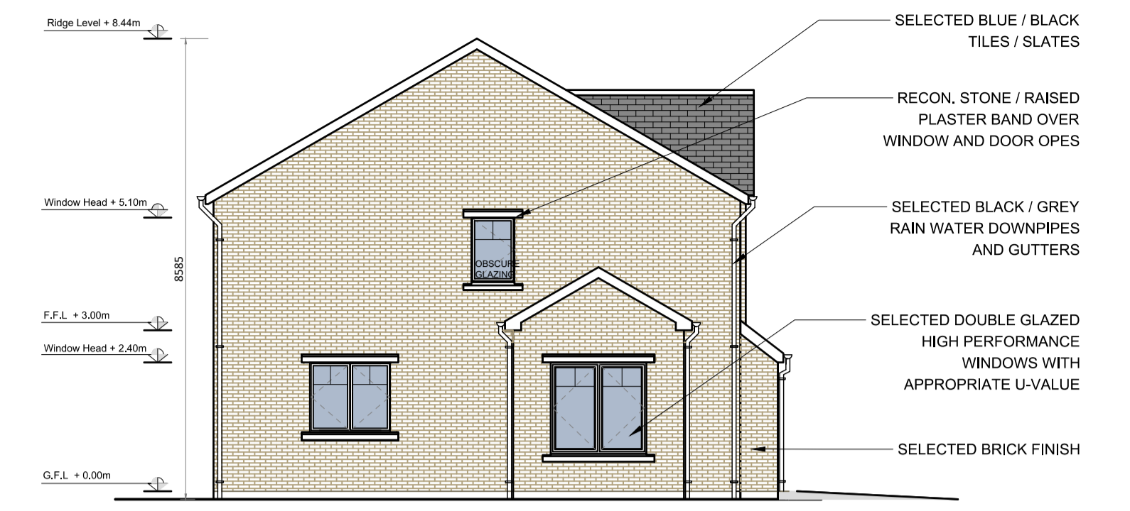
SIDE ELEVATION (UNITS134-137 (handed) /150-153) SCALE 1:100 @A1
